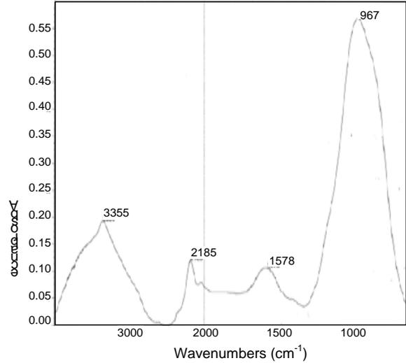
Fig. 3 FTIR spectrum of silicon carbon nitride film
